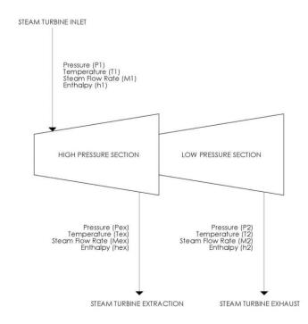
Whether completing a performance calculation on an iso-cooled compressor, sidestream compressor or extraction turbine, performance calculations are best completed section by section. And, the OEM should provide sectional performance curves as well as the overall curves.
