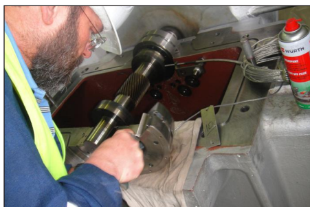
Figure 5: Routine field inspection of a Cooper MSG fuel gas compressor for Electrocentrale Bucuresti, Bucharest, Romania.
