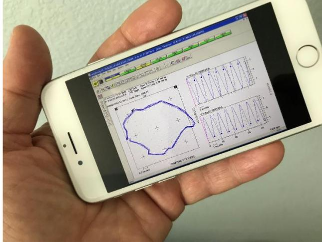
Figure 3. Tying vibration with aerodynamic performance can be very helpful in determining the root cause of the vibration. For example, higher than normal synchronous vibration in conjunction with poor aerodynamic efficiency can mean a dirty or fouled compressor and all that is needed is on line washing to correct the situation.
