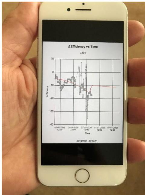
Figure 4. Turbomachinery health is best assessed by trending and forecasting and collectively assessing: delta efficiency (deviation from ideal), vibration, bearing temperatures, balance line delta P, seal operating data and oil analysis.
