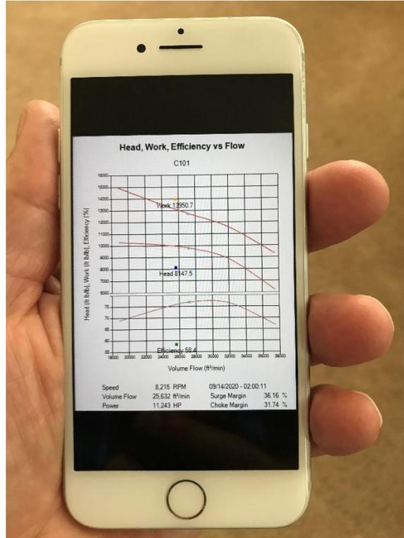
Figure 2. In addition to knowing where the compressor is operating on the curve, knowing the surge margin, margin to choke and work input can be very helpful. Work input is a good indicator of the quality of the data being measured.
