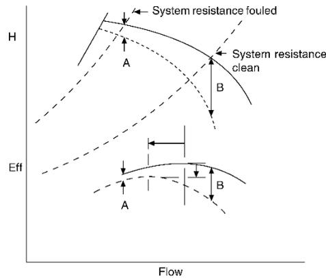
Figure 5. Effect of fouling on compressor performance curves and system resistance curves.
