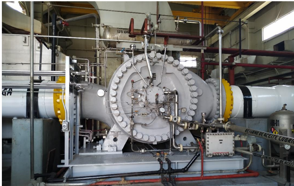
Rolls Royce – Cooper RF2BB-36 compressor
